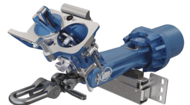
HYBRID DAC FOR LOCOMOTIVES SCREW COUPLER MODE
