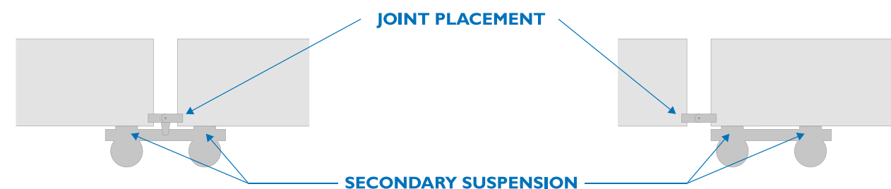
FIGURE 1. JACOB'S BOGIE AND SEMI-TRAILER JOINT.
